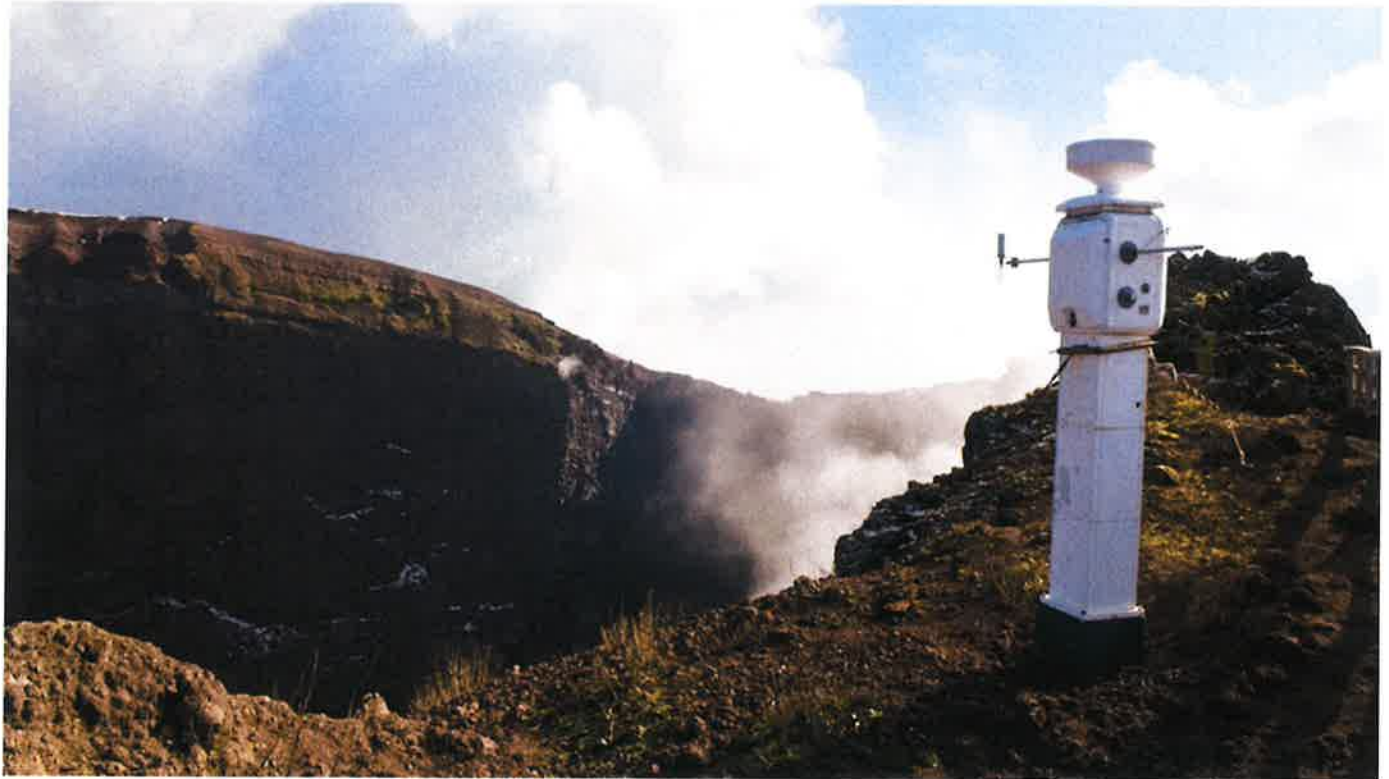
Image 1. A seismological earthquake monitoring station on volcano Vesuvio in Italy. These earthquake monitors send data about ground movements to a central station. Photo: angie7/Getty Images tk
